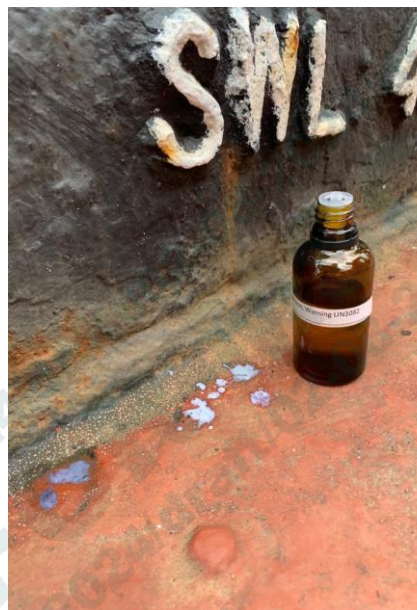
Checking out of AgNO3 solution at the openweather deck for determining of sea-salt content
