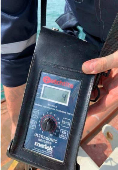
HOLD No2, USWT measurements
