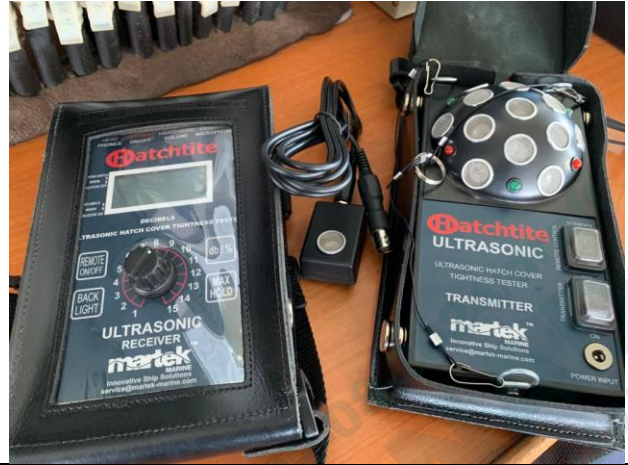
General view and testing of the Ultrasonic transmitters before inspection
